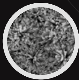
SEM magnification X2000: clear uniform crystalline structure of SBTC® type
