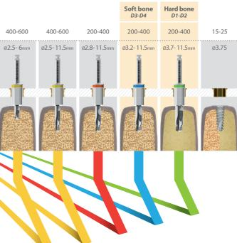
This Protocol shows an example of a Drilling Protocol for an Implant of 11.5 Millimeter Length.
