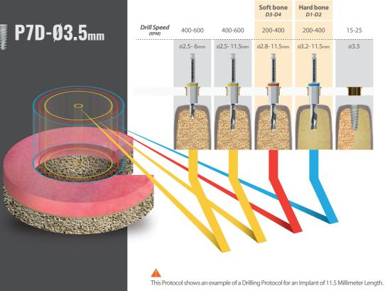
Regardless of the Implant Length being drilled, the First Drill, also referred to as Pilot Drill, will always be the Ø2.0/2.5 L6 drill.
