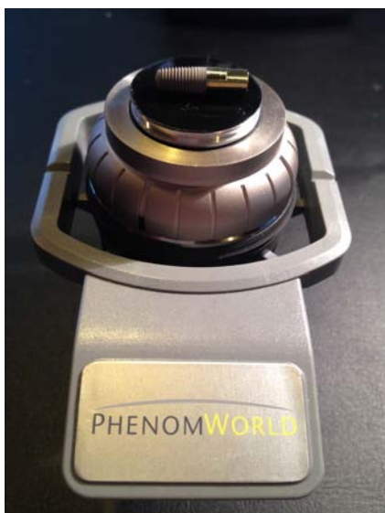
Fixed implant (example) on the sample holder
